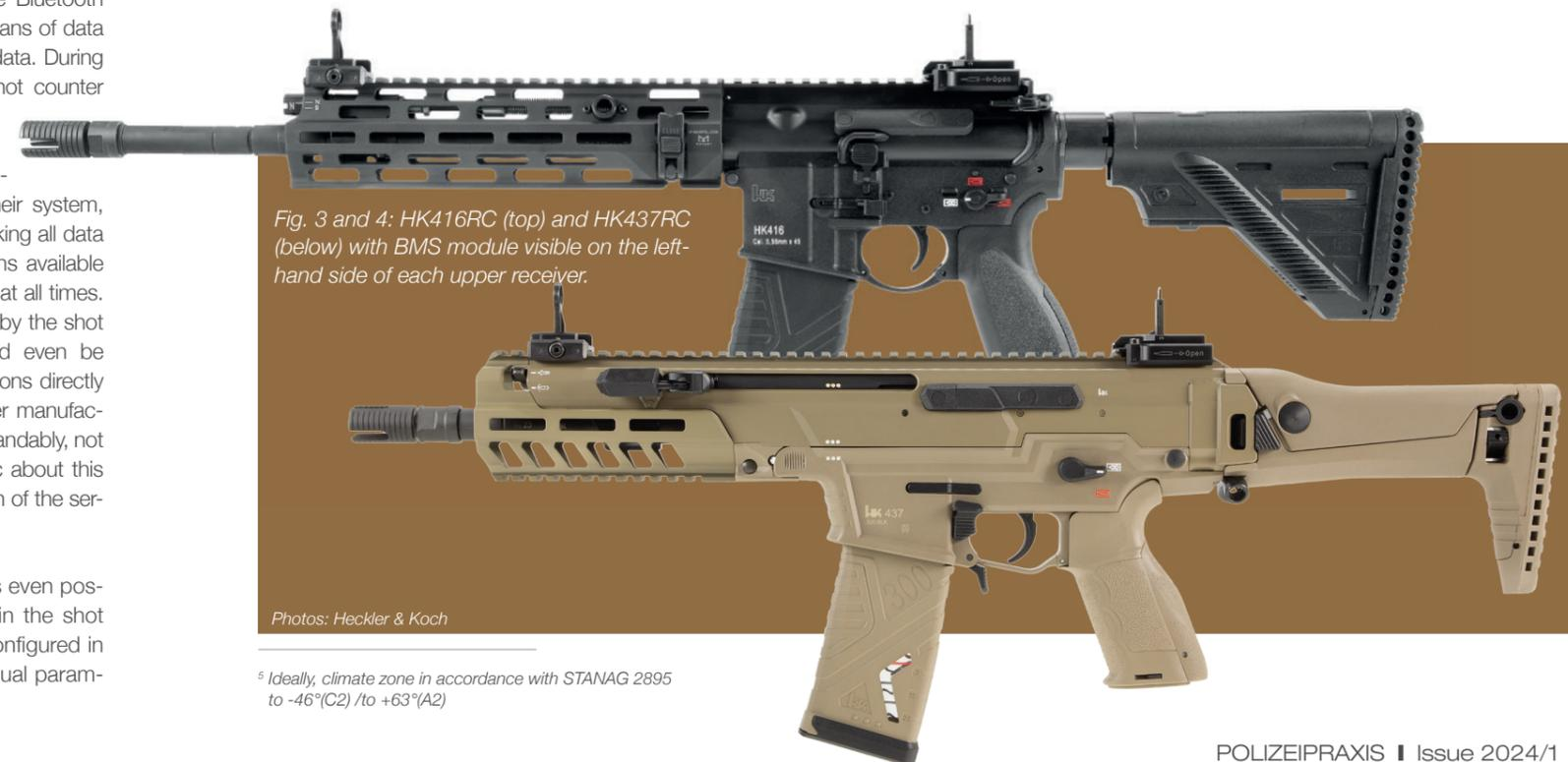
Fig. 3 and 4: HK416RC (top) and HK437RC (below) with BMS module visible on the left-hand side of each upper receiver.
