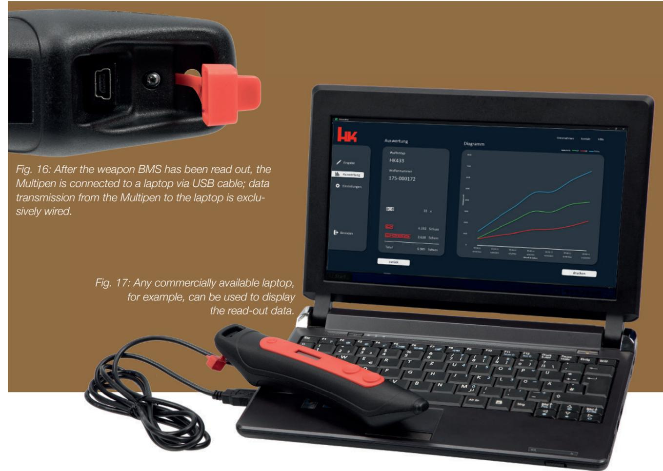
Fig. 16: After the weapon BMS has been read out, the Multipipen is connected to a laptop via USB cable; data transmission from the Multipipen to the laptop is exclusively wired.
