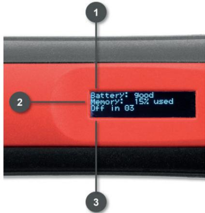
Fig. 13: The following can also be displayed: the battery charge status (1), the amount of internal Multipipen memory used as a % (2) and the time remaining until the Multipipen switches off automatically to save power (3).
