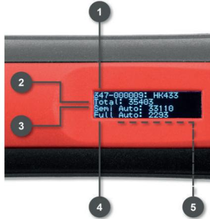
Fig. 12: After the readout process, the following is displayed: the serial number starting with the HK weapon code for the model, followed by the individual number for the weapon and the model name (1), the total number of all fired rounds recorded (2), broken down into the number of movements of the bolt group/slide caused by single fire (3), sustained fire (4), followed separately by the bolt group/slide releases from the rearmost bolt group/slide position (5)<sup>9</sup>.
