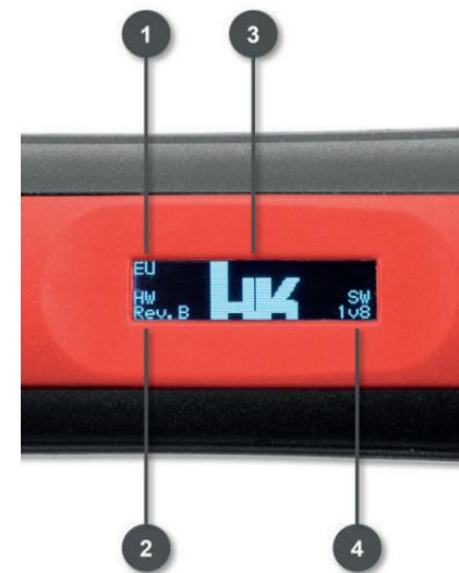
Fig. 10: Multipen display – the "welcome screen." After switching on, the following are displayed: region code (1), Multipen hardware version (2), Heckler & Koch logo (3) and the software version currently installed (4). Users can switch between screen views by pressing a button on the Multipen.
